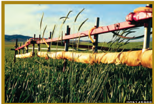
Various types of wiper devices can be purchased or built to mount to ATVs, tractors, or other vehicles. These wipers allow herbicide to wick out onto the surface, where it is applied directly to target vegetation at a set height.
