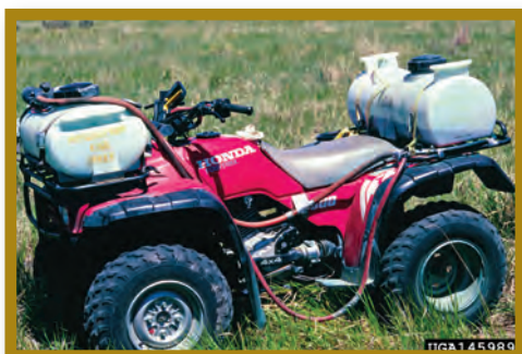
An ATV-mounted tank with a spray gun is useful for spot-spraying scattered plants across large areas of land. ATVs can also be outfitted with boom sprayers for spraying patches of herbaceous vegetation.
